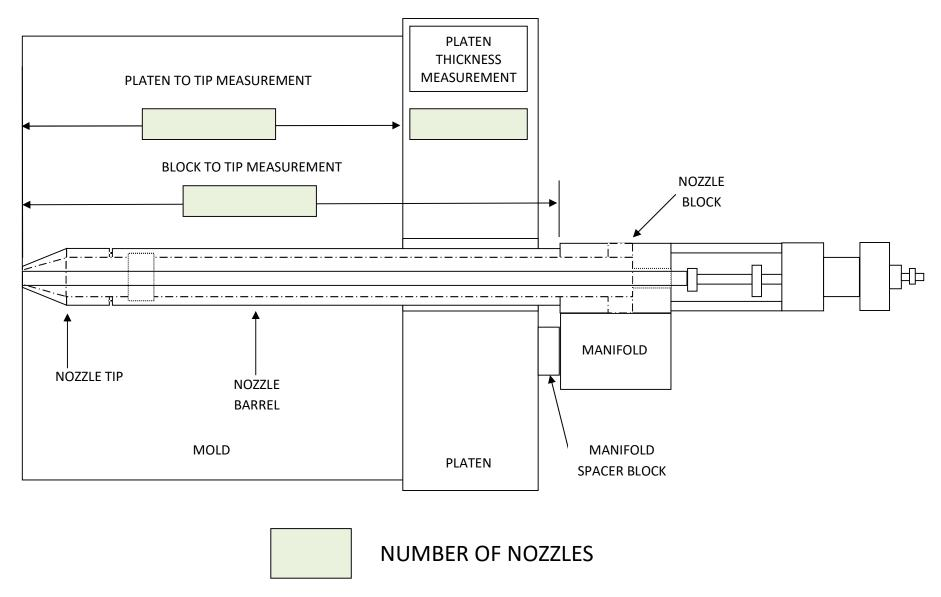
PROVIDE DIMENSION. FOR PLATEN TO TIP MEASUREMENT (PTD) (MOLD SEAT DEPTH) THE PLATEN THICKNESS MUST BE ALSO PROVIDED. FOR BLOCK TO TIP DIMENSION (BTD) THE PLATEN THICKNESS IS NOT REQUIRED
